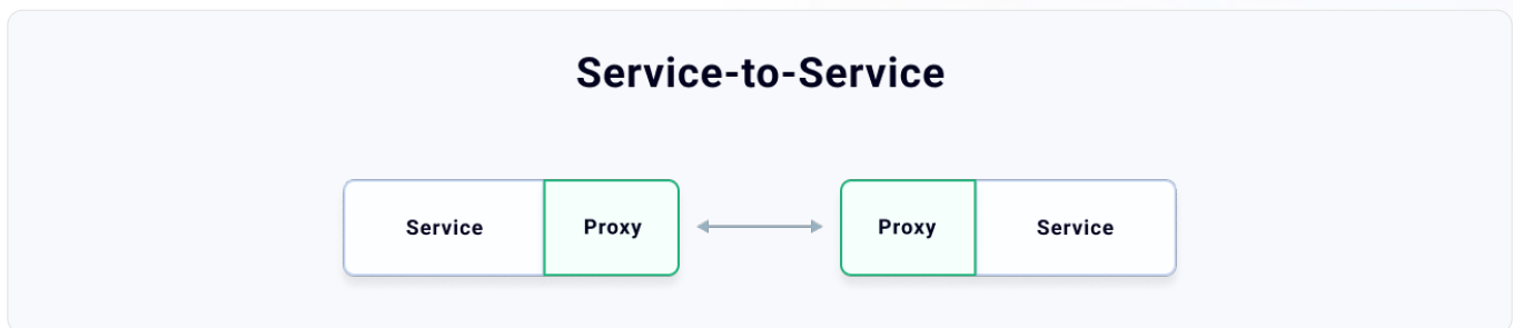
Figure 1: Service-to-service communication example – notice the “sidecar” characteristic of this option
